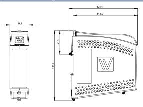
**Dimension W x H x D**  $34 \times 123 \times 121 \text{ mm} (1.33 \times 4.84 \times 4.76 \text{ in})$
