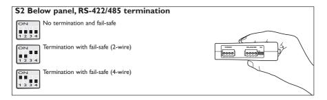
Note! DIP-switch alterations are only effective after a power on.
