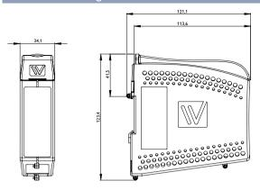
**Dimension W x H x D**  $34 \times 123 \times 121 \text{ mm}$
