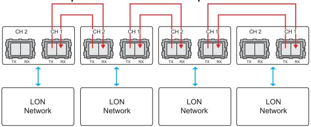
The data is transferred via the fibre optic network to the serial ports of all units. If LRW-102 is connected to two optical fibre links (mid unit) converted data will be transmitted in both directions, via both CH 1 and CH 2. With only one optical fibre link (end unit) converted data will be transmitted in one direction, via CH 1 only. Data received from one LRW-102 optical fibre port will be repeated through the other optical fibre port and it will also convert the frame to serial data.
