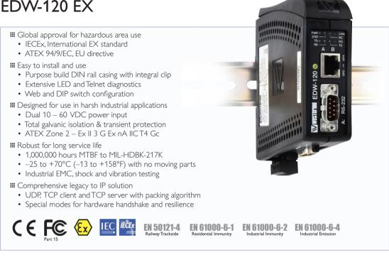
The EDW-120 EX is an ATEX certified dual Ethernet converter designed to allow RS-232 serial devices to communicate via TCP/IP Ethernet networks. DIP switches can be used for configuration of Ethernet port settings if required, and the password protected web interface is used for all other settings. Diagnostic information can be accessed via a Telnet session with more basic information offered on LEDs.
