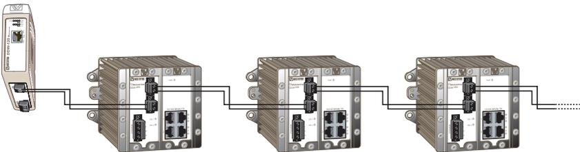
The default configuration of the units allow for an Ethernet extension to be made. Connect DSL 1 to DSL 2 on the following units to obtain a chain of linked units.
