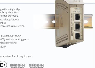
The SDW-550 is an unmanaged 5 port industrial Ethernet switch designed for easy use in heavy duty industrial applications. The unit supports 802.1Q long packets which allows all standard industrial Ethernet protocols to be used.
