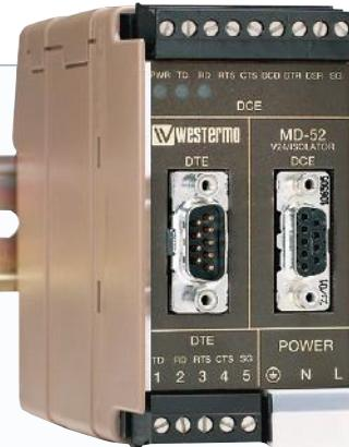
The MD-52 is a RS-232 isolator allowing RS-232 systems to be connected where there is a need to isolate interfaces from each other. The serial interfaces are standard RS-232 configured as DCE and DTE creating a simple installation.
