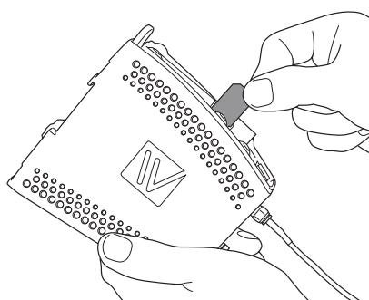
It is necessary to have a GSM subscription from a network operator. They will provide you with a SIM card that should be mounted in the SIM card holder. The SIM card holder is located under the top lid of the unit.
