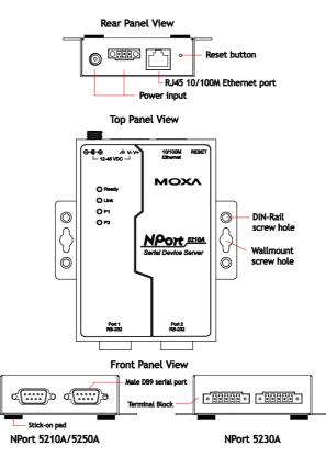
**Reset Button**—*Press and hold the Reset button for 5 seconds to load* factory defaults: Use a pointed object, such as a straightened paper clip or toothpick, to depress the reset button. This will cause the Ready LED to blink on and off. The factory defaults will be loaded once the Ready LED stops blinking (after about 5 seconds). At this point, release the reset button.
