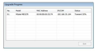
Once the firmware has been successfully written onto the unit, click **Exit** to close the Upgrade Firmware window. MGate Manager will automatically execute a Broadcast Search for all MGate MB3000 units on the LAN. Your MGate should reappear in the list of units.
