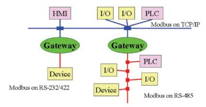
Ordinarily, Modbus TCP and Modbus ASCII/RTU are unable to communicate with each other. However, with a Modbus gateway in between the Modbus serial network and the Modbus Ethernet network, TCP masters are able to communicate with serial slaves, and serial masters are able to communicate with TCP slaves.
