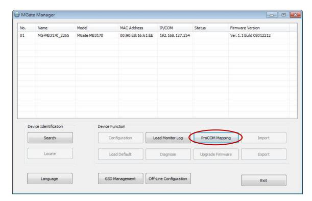
On the ProCOM mapping dialog box, you can map up to four ProCOM functions for each Modbus gateway to your PC's COM ports. The driver will generate virtual COM ports on your PC to connect to the selected MGate MB3000s over the network.
