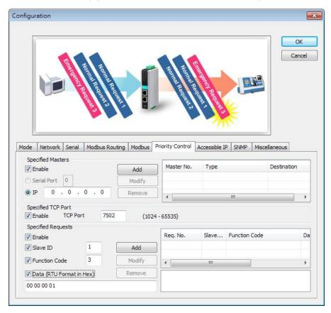
Priority control is designed for requests that are sent to Modbus RTU/ASCII slaves. Since Modbus RTU/ASCII slaves cannot handle multiple requests, the Modbus gateway must send each request individually and wait for the response before sending the next request. As requests stack up, the response time can suffer. This can cause problems for certain critical requests that require an immediate response.
