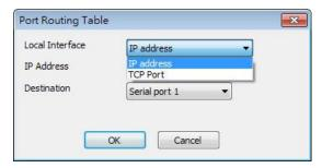
For example, you could assign TCP ports 2001 to 2004 to serial ports 1 to 4, respectively. When the gateway receives a Modbus request designated for TCP port 2001, it will forward the Modbus request to serial port 1 directly. Similarly, if it receives a Modbus request designated for TCP port 2004, it will forward the Modbus request to the serial port 4 directly.
