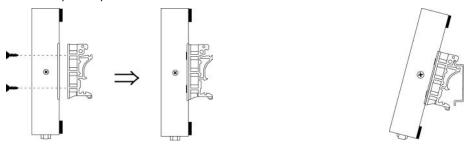
**Mounting on the wall:** You will first need to attach the mounting plates to the unit. Place four screws in the wall and slide the unit onto the screws as shown.
