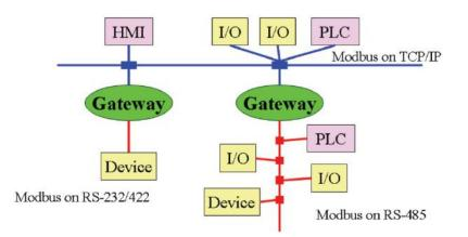
Ordinarily, Modbus TCP and Modbus ASCII/RTU are unable to communicate with each other. However, with a Modbus gateway in between the Modbus serial network and the Modbus Ethernet network, TCP masters are able to communicate with serial slaves, and serial masters are able to communicate with TCP slaves.
