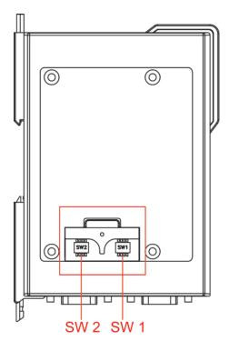
The DIP switches are located beneath the DIP switch panel on the side of the unit.
