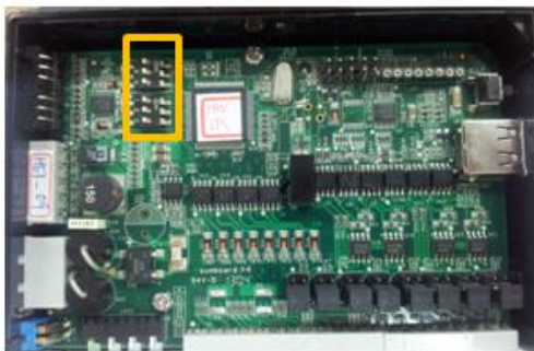
Pull High/Low DIP switch settings for the RS-485 Port
