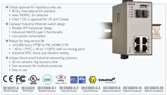
Lynx 106 EX is a layer 2 managed industrial Ethernet switch, powered by the Westermo WeOS network operating. Independently tested for IECEX and ATEX by Baseefa, as well as Class 1 Division II by FM approval, Lynx is the perfect solution for hazardous area applications in any part of the world.
