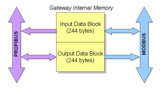
Input refers to the dataflow from the Modbus device to the PROFIBUS master. More specifically, it means the gateway will read the Modbus device's data and store in its input memory area. And the PROFIBUS master will
