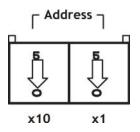
Before communication, you must assign a slave ID to the PROFIBUS slave, If you would like to assign an address between 0 to 99, you need to change the rotary switch to the desired address. If you would like to assign an address which is over 99, you must set it in the MGate utility.
