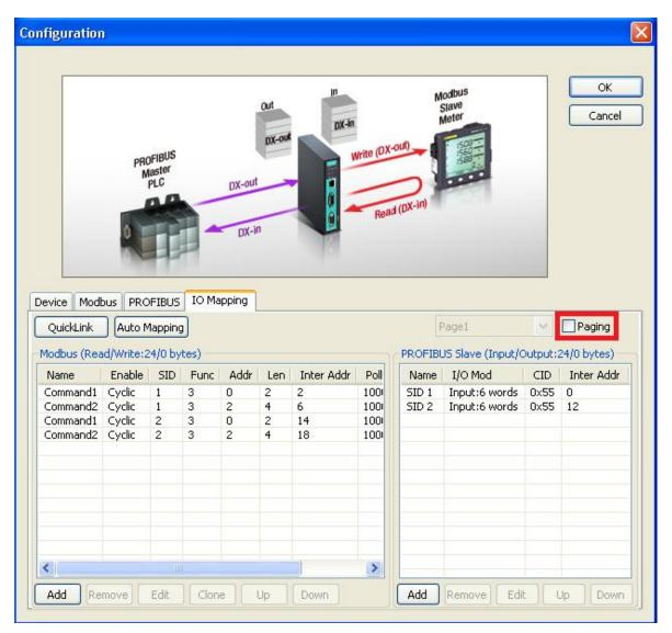
If you want to exchange data over 244 bytes, you can select the **Paging** checkbox to enable the page function, so the utility will insert two I/O word modules into the starting location of the input/output memory bank for separate page functionality. Basically, because one I/O module supports 244 bytes only, the paging function can be used to break through this limit. The maximum of input/output memory size is up to 7744 bytes respectively.
