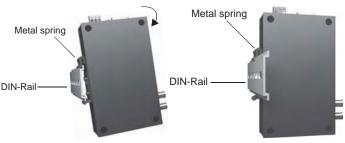
To remove the ICF-1170I series from the DIN-Rail, simply reverse Steps 1 and 2 above.
